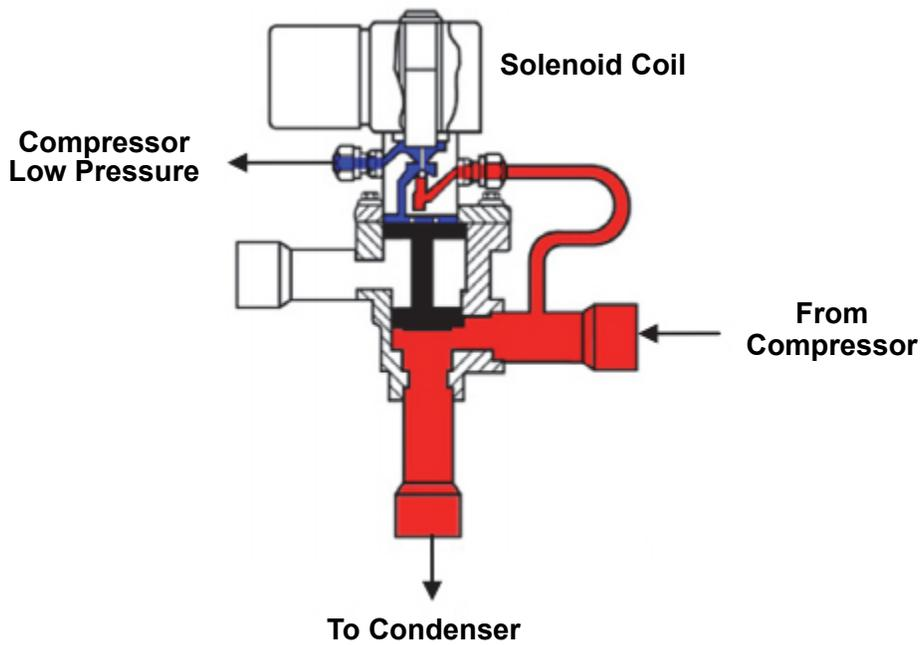
Figure 2.6 3-way Valve (HGS) Heat & Defrost Mode
