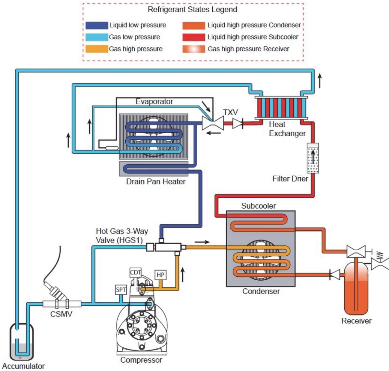
**Figure 2.8 Refrigeration Circuit - Heat and Defrost**
