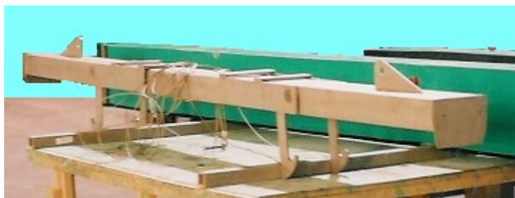
Stop Log Lifting Beam
