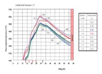
Fig. 4: Variation of FEGT for hard coal with different emissivity values **E** [1]
