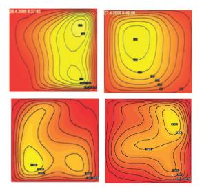
Fig. 6: Temperature distributions in 200 MWel hard coal, opposite wall fired (above) and in 800 MWel lignite, tangential fired (below)
