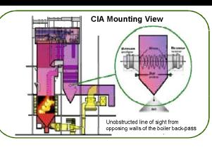
Carbon in Ash offers Real time (24X7) Online monitoring of un-burnt carbon based on Non-Extractive methodology!
