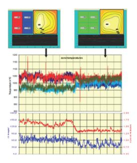
Fig. 12: Effects of temperature balancing on 4 zone temperatures above, O2 (red) and CO (blue), 800 MW lignite
