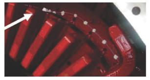
Fig. 2: Sensor on the end windings cap
