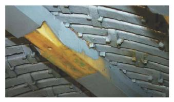
Fig. 1: Insulation crack and abrasion between end winding support elements
