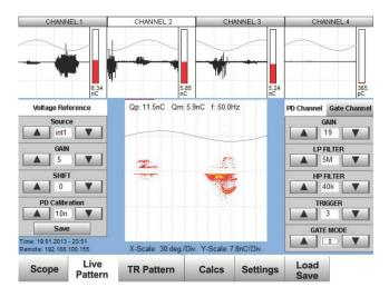
Fig. 11: Real Time Live phase resolved partial discharge Pattern
