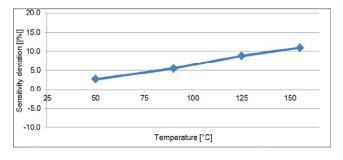
MC-Monitoring Fibre Optic acccelerometer 2
