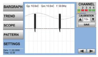
Fig. 8: Automatic pulse level detection
