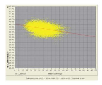
Fig. 13: Net efficiency vs. temperature imbalance, 660 MWel hard coal
