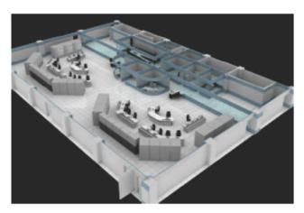
Fig 1: Typical MCR for 700 MWe NPP
