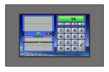
Operator Panel OP7 is a color touch-panel with an LCD display and a graphic safety Status Information Panel. It has an Ethernet interface that can be used for Remote Access!
