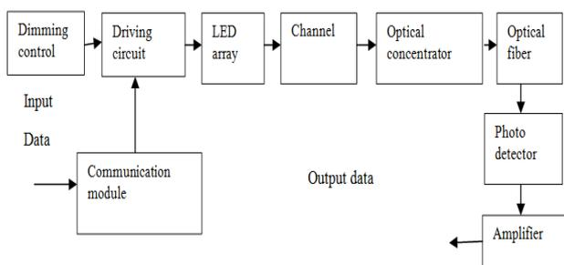
Fig.1: A block diagram of VLC
