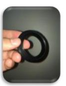
When installing the Linear Lens Hub, if the gasket is serviceable, reuse it; If the gasket is damaged, replace it. The gasket sets at an angle when installed properly around the sloped surface of the outer flange of the Linear Lens Hub.
