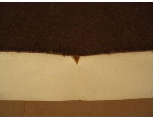
Knit line and V-groove close-up (after conditioning)
