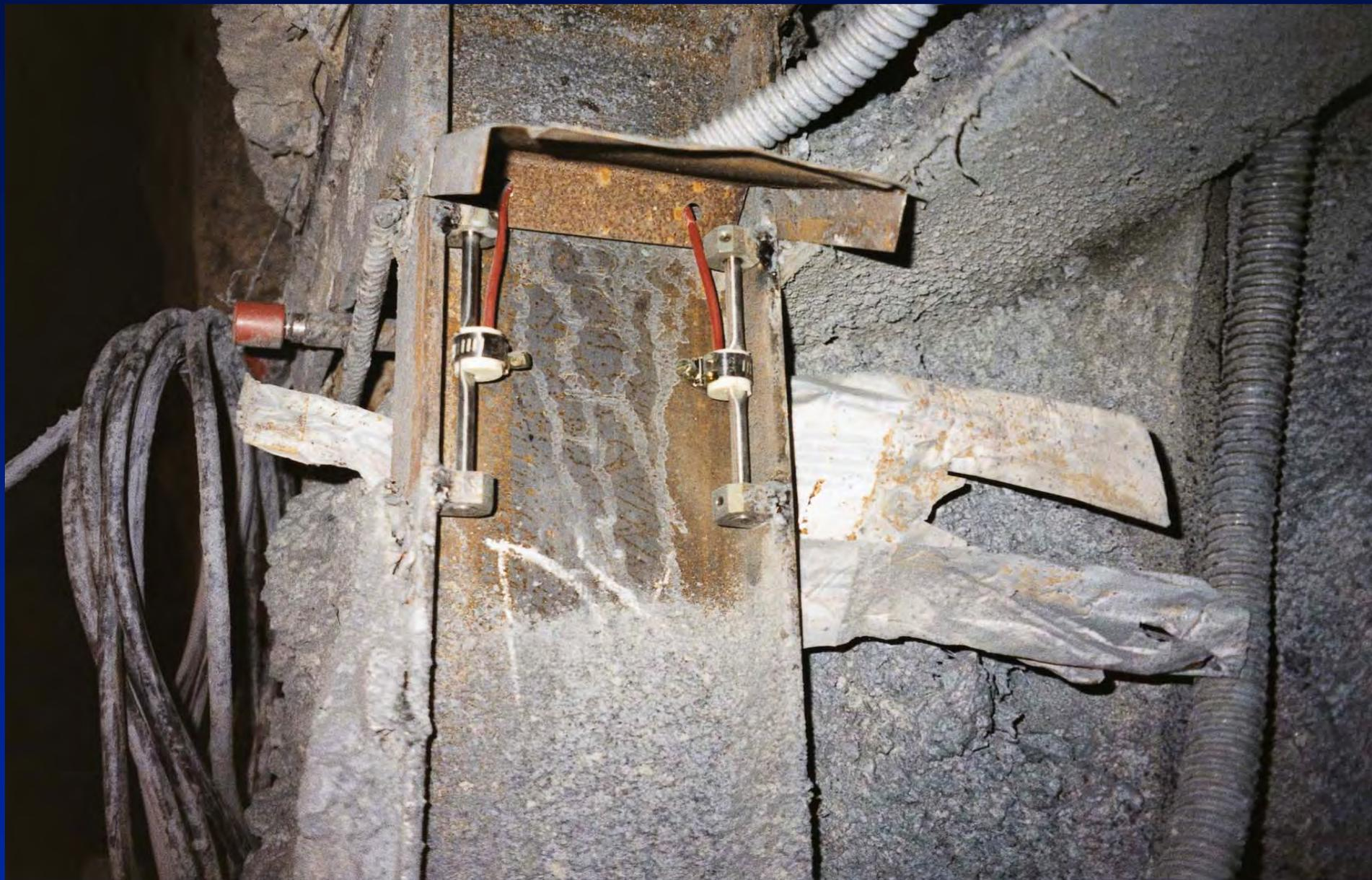
**Strain gauges a corda vibrante**
