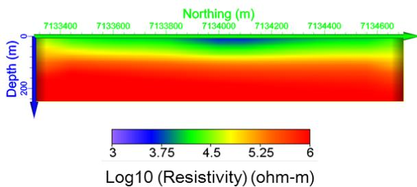
**Figure 3.** The cross-section (at 558800 m easting) of reconstructed conductivity results obtained after inverting out-of-phase data over dike zone.
