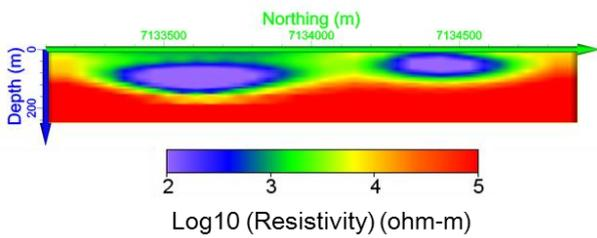
**Figure 2.** The cross-section (at 557250 m easting) of reconstructed conductivity results obtained after inverting out-of-phase data over kimberlite zone.
