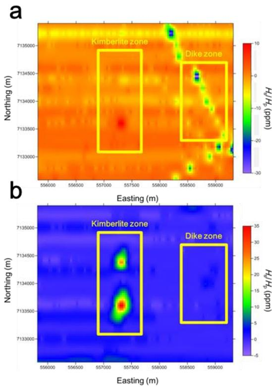
**Figure 1.** The data maps of (a) in-phase and (b) out-of-phase components at 900 Hz. The yellow rectangles indicate the region where the data sets were inverted.
