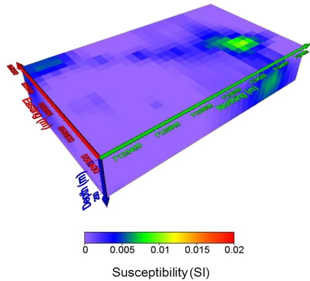
**Figure 4.** The reconstructed susceptibility results obtained after inverting in-phase data over dike zone.
