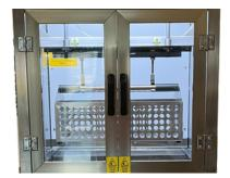
Security switch attached, tempered windows for top level EHS compliance
