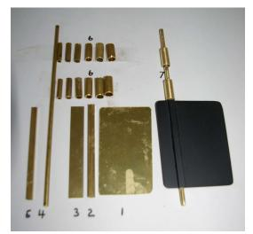
The rudder blade is made up from items 1, 2 and 3 shown. Items 1 and 3 are brass sheet, and item 2 is square section tube. They are soldered together in the same way that Garth and Steve made their open rudders.
