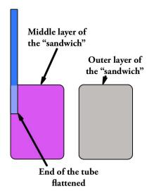
Figure G. A rudder using brass tube as a rudder post.
