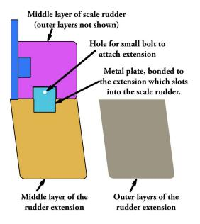
Figure A Constructing a rudder extension.
