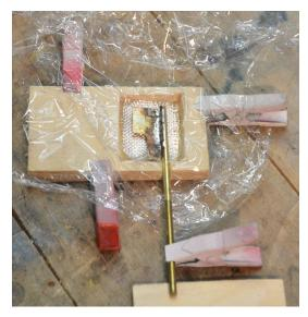
Figure K. The mould ready for the epoxy. In this photo a second piece of wood is used for the base of the mould and the two clamped together.
