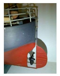
Figure E The completed rudder on Steve's Clyde Puffer.
