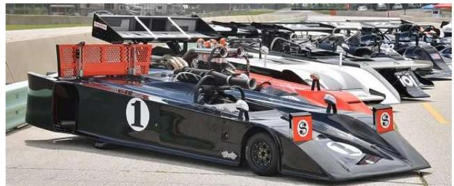
*The Mk1 Shadow with its air brakes deployed at the front of a row of later Shadows. The hybrid wing/radiator of the orange developed version behind towers over both chassis.*
