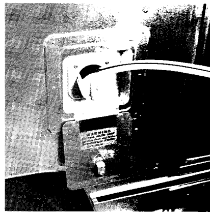
Water Tank Fill Spout
