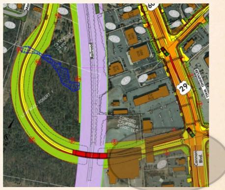
This is a <u>real example</u> of how major changes may occur. In the first design, the brown "L" shaped building was planned to be barely impacted along the existing road frontage. Once the design-build team came in, they changed the design and the property was <u>totally</u> damaged. The new road now goes through the middle of the property. At no point during any of the preliminary discussions did the land owner ever think this would happen to his property.
