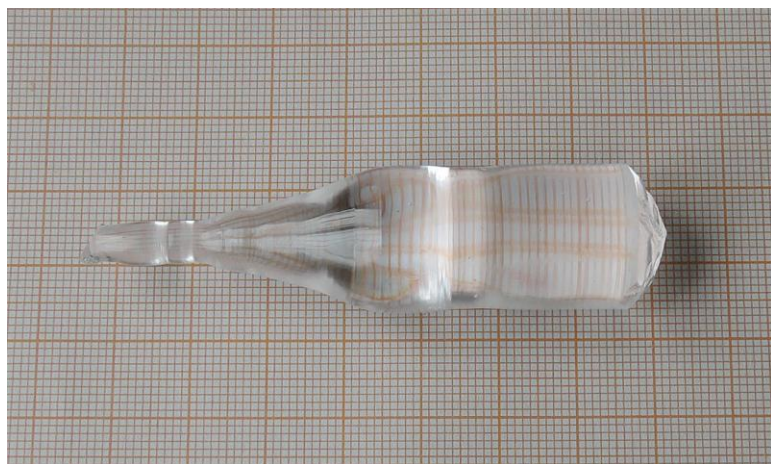
Figure 1. The \text{Ca}_3(\text{BO}_3)_2 single crystal grown by Cz method along crystallographic c axis
