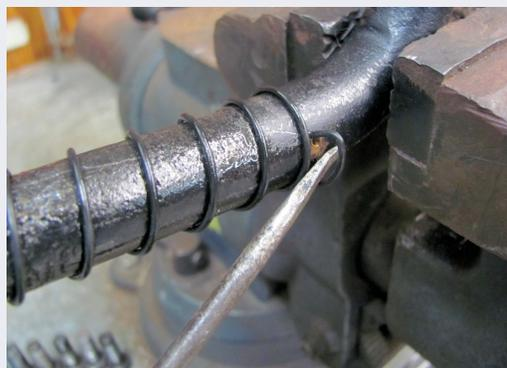
With the new crank spring fitted, slide the starting crank into the nose of the engine pan and re-fit the ratchet with its pin and cotter pin.
