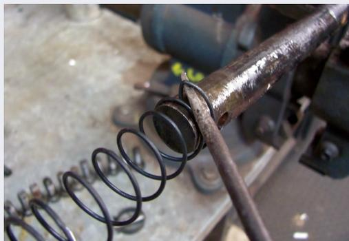
Finally, lift the prong and slip it into the hole to secure the spring on the starting crank. Be sure the bent end of the spring is fully inserted into the hole.
