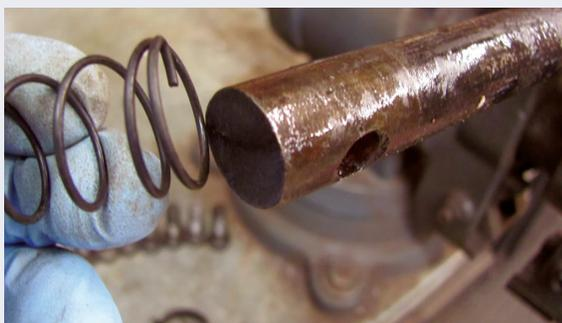
The tiny hole is first located near the bent end of the starting crank. Using a small twist drill, clean out the hole which goes part way into the shaft.
