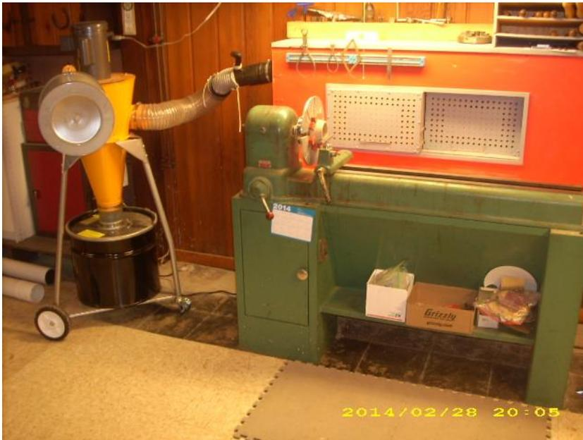
Ken Urtel uses an Oneida Air "Mini Gorilla" (having 1.5 hp and 600 cfm capacity) in his shop. This is a high capacity portable system with a quick connector which can be used on individual machine or short run manifolds to multiple machines within the shop. Ken hooks this unit to his wood lathe via a single port connected to two homemade collector boxes placed side by side to cover the length of the lathe bed.
