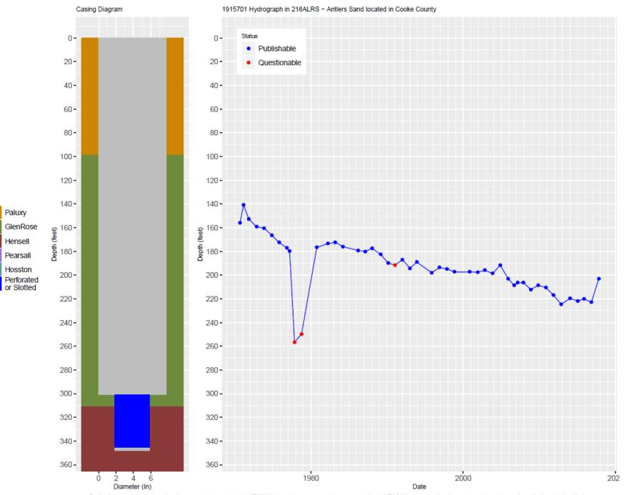
The Aquifer layers shown in the casing diagram were developed using the NTWGAM. In certain cases, assumptions used to develop the NTWGAM can cause well casing and screen intervals to not align well with modeled aquifer layers.
