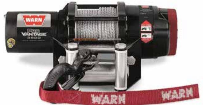
For vehicle recovery or to raise and lower snow plow blade. 3,500 lb. (1,588 kg) capacity, reversing with free wheeling feature. Comes with 40' (12 m) cable with 30' (9 m) nylon strap. Safety switch disables winch unless ignition is on. A 4,500 lb. (2,041 kg) winch is standard on Conquest models.
