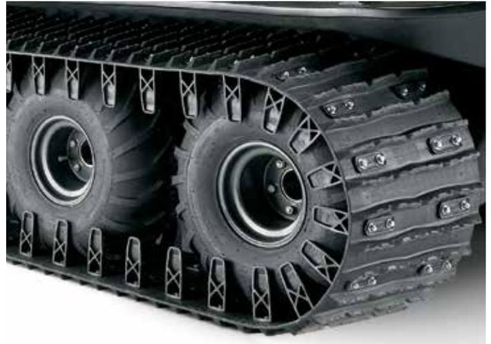
Heavy duty 18" (457 mm) wide rubber track provides optimum flotation with minimal ground pressure. Exceptional traction. Lightweight durable construction and low rolling resistance ensures smooth, quiet operation in difficult terrain conditions. Available with or without axle extensions.
