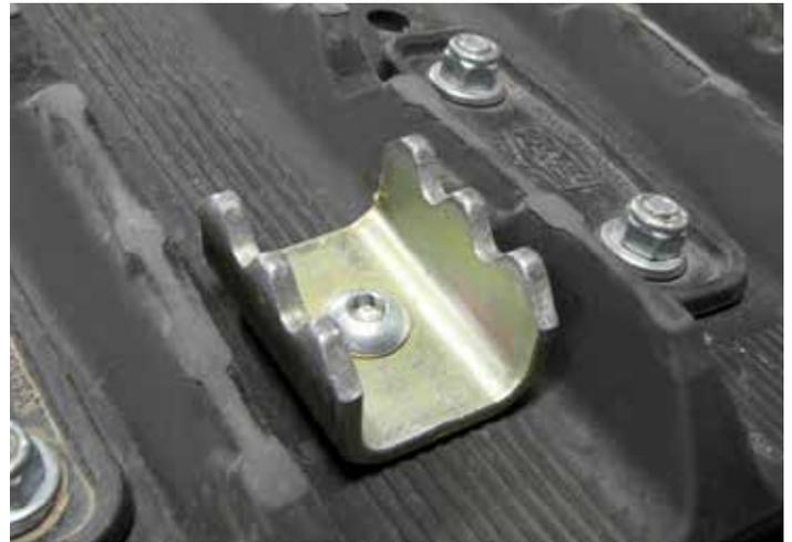
Steel cleats increase traction on ice and hard-packed snow. Available for all track configurations.
