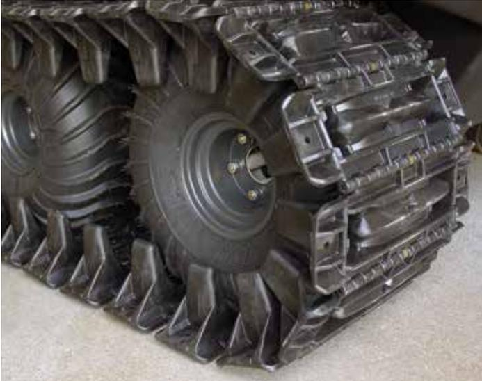
General purpose, mud & snow, segmented plastic track ranging in width from 13" (330 mm) to 18" (457 mm). Segments are light weight, easily replaced and formed from thermoplastic rubber compound to withstand impact and reduce wear. Comes with axle and stud extenders, fits over 24" tires.
