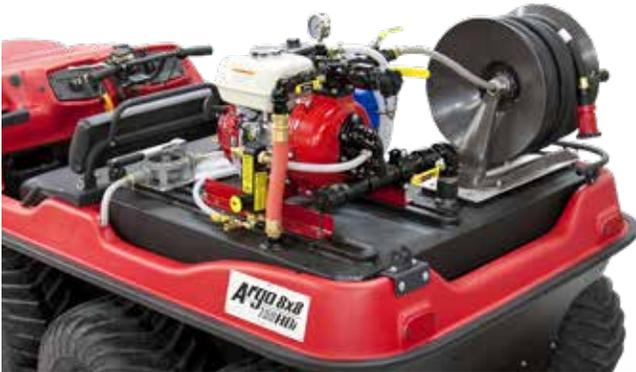
Custom designed to fit into the rear compartment of any 8x8 Frontier or Avenger; the 80 gal. (303 L) fire suppression unit holds 75 gal. (284 L) of water plus a 5 gal. (19 L) foam cell. Packaged with a Honda engine, two-stage CET centrifugal pump, 100 ft. (30.5 m) of hose and forestry nozzle. Compatible only with standard backrest and rear floor pan removed.
