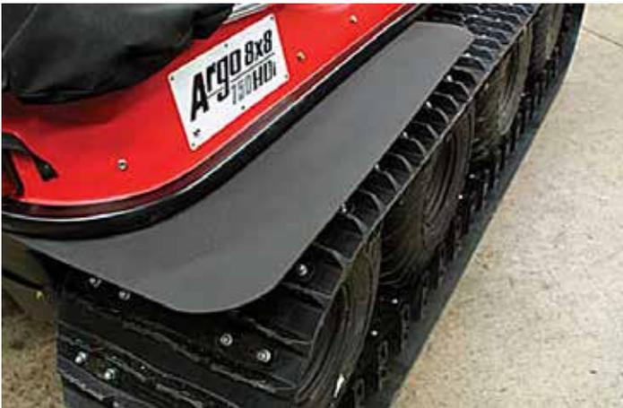
Deflects snow and mud. Stay dry and clean when navigating through challenging terrain. Easy to install.
