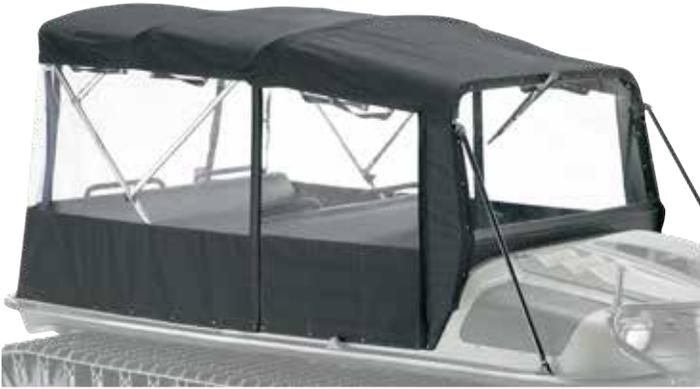
Protects all occupants or cargo from outdoor elements. Converts from a full enclosure to bimini top by removing all sides. When not in use, the top is easily removed or folded down and protected with the included boot cover. Requires fold-down windshield.
