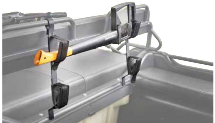
The utility bracket consists of two "rugged gear" utility hooks and a barrel holder. It is an ideal way to safely secure objects such as shovels, fishing rods, paddles, etc. to the outside or inside of your ARGO.
