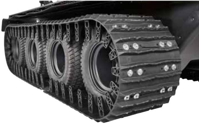
Xtreme duty 18" [457 mm] wide rubber track with UHMW-PE guides, reinforced turf tire and rim provides optimum flotation with minimal ground pressure. Designed for use with Conquest models, this track offers quiet operation, superior wear and durability in difficult terrain.
