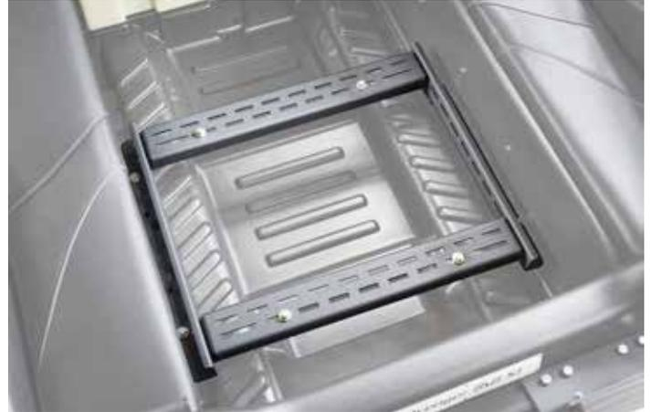
Quick change universal mount. The sub frame holds up to 750 lb. (340 kg); bolts directly to main chassis offering a secure structure for third party equipment.
