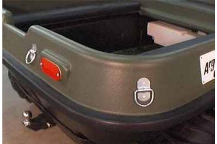
Six rings mount near the rear compartment (four rings for 6x6 models).
