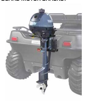
This one-piece bracket mounts to the bumper and rear receiver hitch bracket. Mounting location is slightly off-center and accepts an outboard motor of up to 9.9 HP for increased propulsion in water. Not compatible with 868-01 Tlre Carrier.
