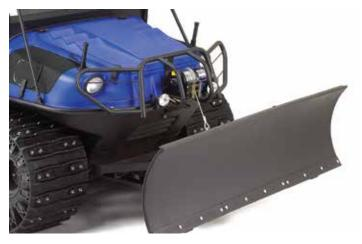
81" (2 m) wide steel blade features multi-angle positions. Attaches to front bearing extension housings. A snowplow will maximize the utilization of your ARGO when the snow flies. Requires the power winch for raise and lower operation.
