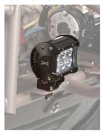
Mounts directly to the brushguard. Provides added illumination in poor visibility due to rain, fog, dust or snow.
