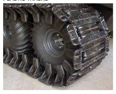
General purpose, mud & snow, segmented plastic track ranging in width from 13" (330 mm) to 18" (457 mm). Segments are light weight, easily replaced and formed from thermoplastic rubber compound to withstand impact and reduce wear. Comes with axle and stud extenders, fits over 24" tires.
