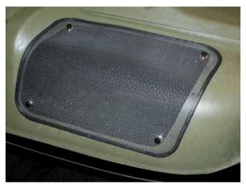
Fastens directly to the air intake to prevent debris from entering the engine compartment. Easily removable.
