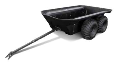
Up to 600 lb. (275 kg) load capacity in a black 6-wheel lower body with ARGO axles and wheels. Complete with 24" (610 mm) or 25" (635 mm) tires. Available for all models.
