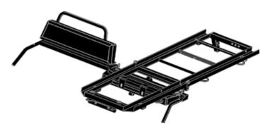
Design to accept either Ferno #9 or Ferno RE 1125 (requires additional basket mount adapter). Fits ARGO 8x8 Avenger Models. Mount adapter can be adjusted for repositioning of front and bench seating. Front bench backrest is folded down when basket or stretcher are deployed. Cannot be used with Suspension Seats or Handrails.
