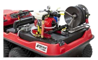
Custom designed to fit into the rear compartment of any 8x8 Frontier or Avenger, the 80 gal. (303 L) fire suppression unit holds 75 gal. (284 L) of water plus a 5 gal. (19 L) foam cell. Packaged with a Honda engine, two-stage CET centrifugal pump, 100 ft. (30.5 m) of hose and forestry nozzle. Compatible only with standard backrest and rear floor pan removed.
