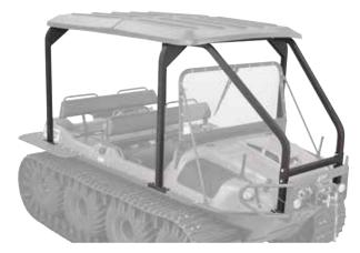
Full vehicle roll over protection complete with two seat belts for driver and passenger. Available for all models with options for seat belts and rear bench (8x8 Models only). Cannot be combined with light bar, suspension seats or standard brushguard.
