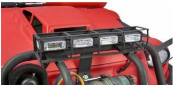
Small size and fully waterproof design make the red and white light Dominator the versatile answer to all your warning and signalling needs. This small but powerful light array is the solution to your unique warning light requirements. Note: Dominator mounts onto optional brushguard.
