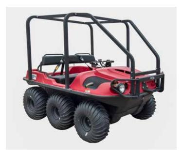
For unpredictable and extreme terrain comes additional protection for the ARGO Frontier 6x6 models. Rollover Protective Structures (ROPS) give you full vehicle rollover protection with two seat belts for driver and passenger safety.
