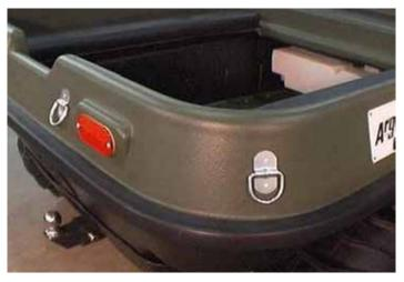
Six rings mount near the rear compartment (four rings for 6x6 models).
