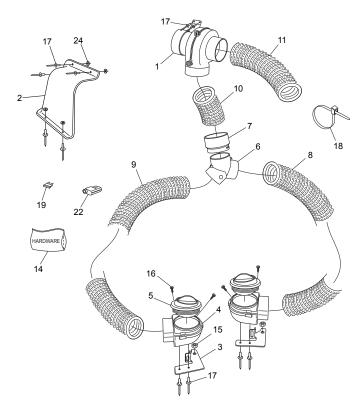
105 CFM fan directing cool air to the service brakes.
