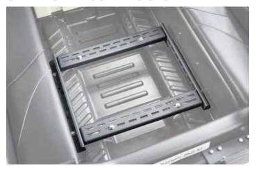
Quick change universal mount . The sub frame holds up to 750 lb. (340 kg); bolts directly to main chassis offering a secure structure for third party equipment.
