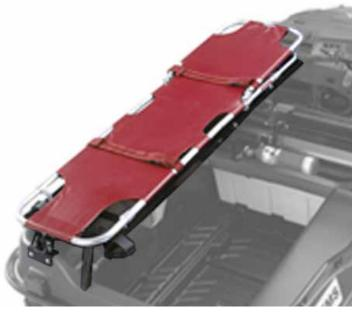
To be used with ARGO Frame Assembly. Cannot be used with Suspension Seats or Handrails.
