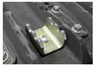
Steel cleats increase traction on ice and hard-packed snow. Available for all track configurations.
