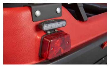
Multi-purpose strobe lights designed for making the vehicle more visible. Super-LED lightheads provide reliable, bright light which will stand up to harsh environments and vibration. 2 x red/white ion (rear) 4 x Vertex red/white with flanges (corners).
