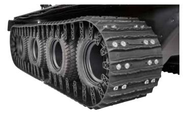
Xtreme duty 18" (457 mm) wide rubber track with UHMW-PE guides, reinforced turf tire and rim provides optimum flotation with minimal ground pressure. Designed for use with Conquest models, this track offers quiet operation, superior wear and durability in difficult terrain.
