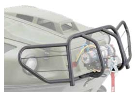
Stylish and functional; body, lights and winch are protected from brush. Offers a mounting location for extra fog lights. Use part# 642-80 if equipped with ROPS.
