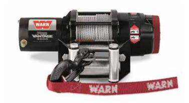
For vehicle recovery or to raise and lower snow plow blade. 3,500 lb. (1,588 kg) capacity, reversing with free wheeling feature. Comes with 40' (12 m) cable with 30' (9 m) nylon strap. Safety switch disables winch unless ignition is on. A 4,500 lb. (2,041 kg) winch is standard on Conquest models.
