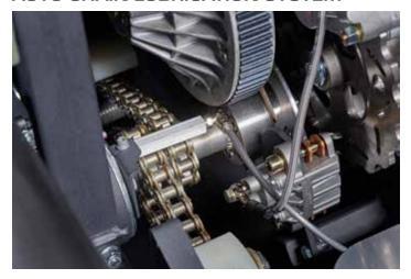
Automates chain lubrication requirements. The system automatically delivers chain lube every 15 minutes of vehicle operation for a total spray time of 5 seconds. A one-hour timer is also available for applications that requires less frequent chain lubrication. Lube system can be manually operated with switch on dash.
