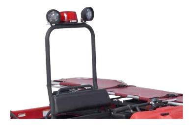
A multitude of options to light up your Responder vehicle. Choose from red and white perimeter strobe lighting, overhead spot lights, front mounted siren/speaker & strobe. All lighting is LED to reduce electrical load.
