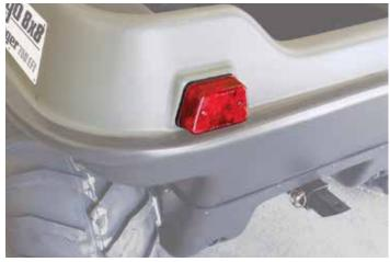
Be seen. Brake/tail lights provide an extra level of safety while trail riding at night. Illuminated when the headlights are on and signals drivers behind you when brakes are applied.
