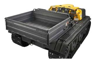
For moving bulk loads over broken terrain, this solid steel dump box handles payloads up to 1,000 lb. (450 kg). Offload easily from the driver's seat using the 14" stroke actuator to top tilt or dump the box (Not for amphibious use). Available for Conquest Series only.
