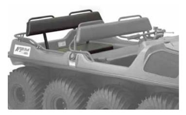
Frame mounted, forward facing rear bench seat provides additional seating for 2 passengers. The bench seat can be removed quickly, without tools, to gain unrestricted access to the rear cargo area.
