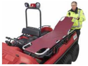
Support structure that provides users with option of adding one revolving light (Whelen L31 red beacon - 850-305) and two spotlights (Whelen PAR 23 LED spotlights - 850-307) in order to aid visibility due to rain, fog, dust, or snow. Note Requires mounting bracket 850-306.
