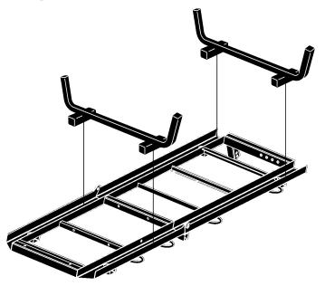
Brackets for basket mount carrier. To be used with FERNO RE 1125 (Accessory# 850-289). Requires Stretcher Mount Adapter (850-300)\* Cannot be used with Suspension Seats or Handrails. Basket required for this carrier is available from FERNO part# RE1125.
