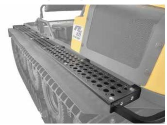
6.25" (160 mm) steel platform runs the full length of the vehicle. Includes a 10" (255 mm) mud flap. Available for Conquest Series only.
