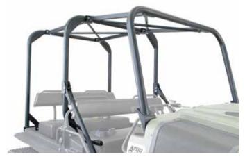
(Conquest Series Only) Driver and front passenger Roll Over Protection Structure complete with seat belts, certified to ISO 5700. Also available in an extended vehicle configuration, up to 4 people when rear bench seat is installed.
