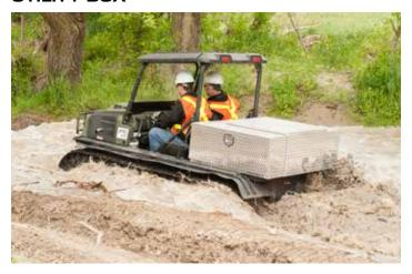
Custom, checker plate constructed of aluminum (.100"), stainless steel T-locks and gaskets. Lift-up lid and rear door include gas shocks and three-point lock. Provides full access to rear cargo area.
