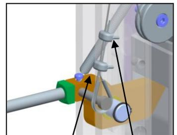
Clamp using wire rope clips (6-2060)
