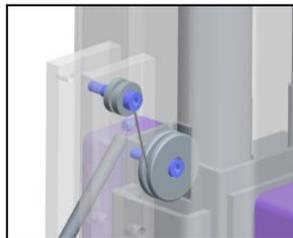
Guide the cable up under the large pulley on the power side.
