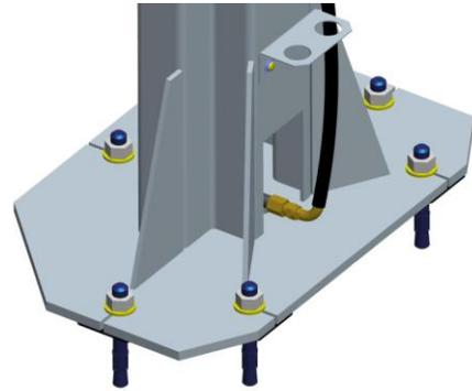
5.13.7 Verify that the entire lift is level both horizontally and vertically to ensure optimum lifting performance. **NOTE: Perform a monthly inspection and torque all anchor bolts to 150 ft-lbs. (203 Nm).**
