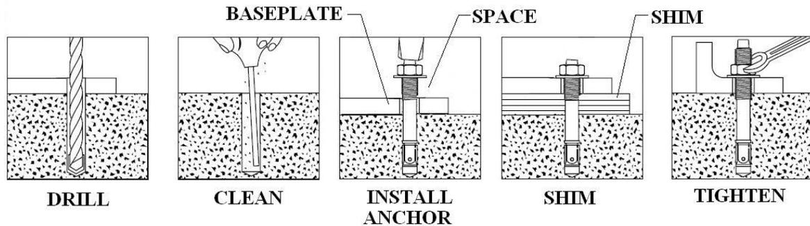
5.12.5 Using a  $\frac{3}{4}$ " concrete drill bit and rotary hammer drill, drill  $\frac{3}{4}$ " holes for the anchor bolts on the high side column. Drill through the concrete floor. (In case longer anchors are required, supplied anchors can be hammered through concrete).
