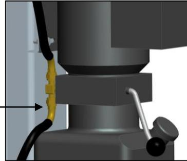
5.10.3 Remove the plastic cap from the bottom of the power side cylinder and connect the short hose to the cylinder.
