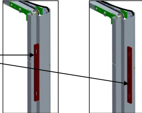
**Note:** Use shims under baseplate to level the column.
