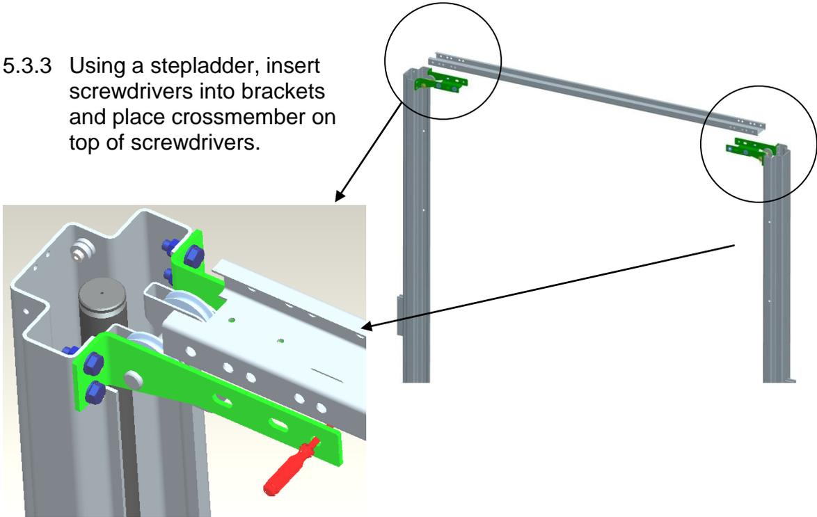
5.3.4 Locate crossmember to the correct holes in the bracket and install fasteners.
