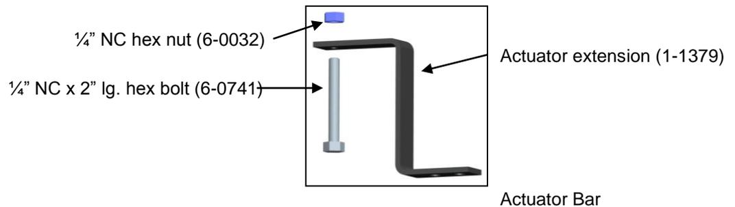
5.14.4 Bolt the Actuator Extension onto the open end of actuator bar.
