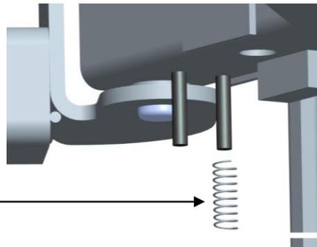
5.7.5 Hammer a spring retainer cap to the end of the arm lock leg.
