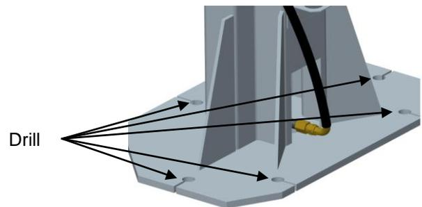
5.12.6 Clean out the drilling dust from the holes and hammer in the anchor bolts until they make contact with the baseplate. **Hand tighten all anchor bolts.**
