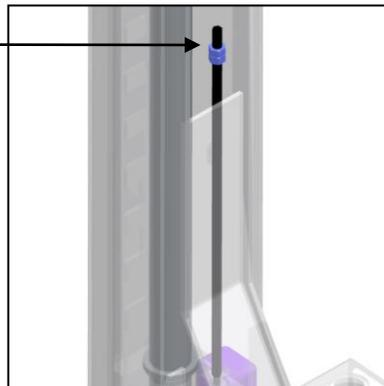
5.5.4 Pull the cable back down on to the carriage bottom plate.
