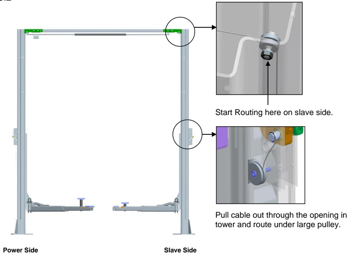
5.8.3 Fix the collar of the safety release cable to the shoulder bolt on the safety dog.
