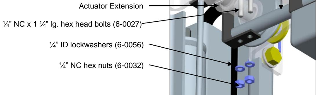
5.14.5 Adjust the 1/4" NC x 2" lg. hex bolt so that the end of the bolt is in contact with the carriage. Tighten the 1/4" NC hex nut on the bolt.
