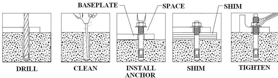
5.13.4 Using a  $\frac{3}{4}$ " concrete drill bit and rotary hammer drill, drill  $\frac{3}{4}$ " holes for the anchor bolts on the high side column. Drill through the concrete floor. (In case longer anchors are required, supplied anchors can be hammered through concrete).
