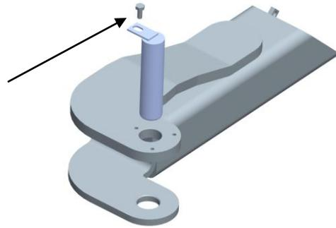
5.6.2 Install the four arms on the carriages by inserting the arm pins.
