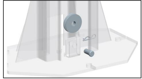
5.5.6 Route equalizing cable around pulley and reassemble the pulley to the base plate. **IMPORTANT – Hitch pin must be installed securely.**
