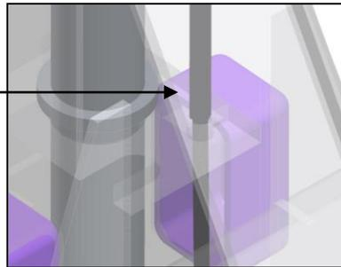
Pass the cable until it reaches the top opening. Tighten a ½"-13UNC nut to the center of the stud, and then **firmly tighten** a second nut up against it using two wrenches.
