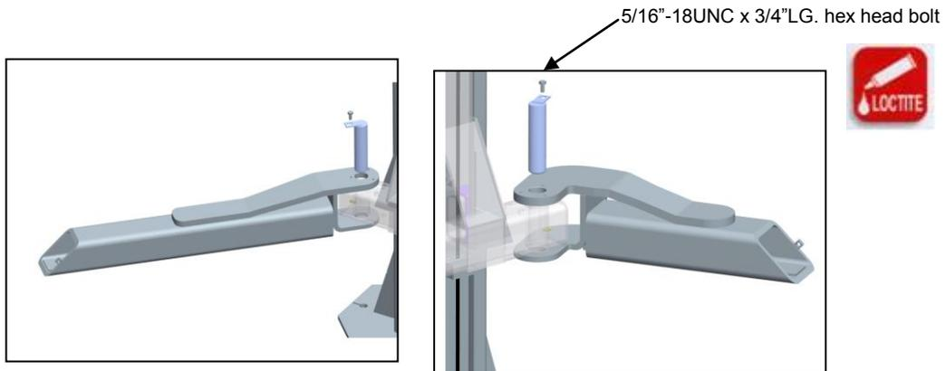
5.6.3 Install Arm Restraint Gear.
