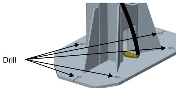
5.13.5 Clean out the drilling dust from the holes and hammer in the anchors until they make contact with the baseplate. **Hand tighten all anchor bolts.**
