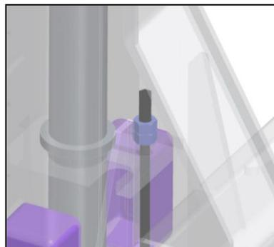
5.5.5 At the bottom of the column, remove the hitch pin, pulley pin and pulley from the base plate.
