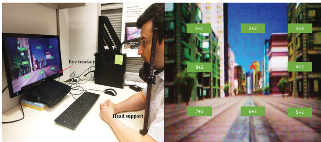
Figure 2. Direct vision environment equipment. Left: Eye tracker Tobii X2-60. Right: The mathematical equations of the task.
