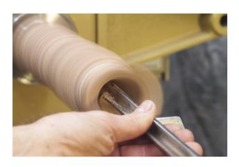
9 The interior of the goblet can be hollowed in several different ways. The generally accepted method for hollowing end-grain is back cutting from the center out toward the rim with either a spindle or bowl gouge. Here I am using a 5/8" fingernail grind bowl gouge. This cut is not a bevel supported cut but more of a scraping cut with the gouge flute rolled over toward the left side of the goblet interior.
