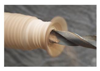
8 I prefer to drill the goblet using a standard 1" metal cutting bit; this removes a lot of material quickly along with the hard to remove center portion. A forstner bit can be used but this leaves you with a flat bottomed hole which I don't like and find harder to round into the bottom of the goblet. The depth of the drilled hole depends on the design and shape of the goblet. Once the hole is drilled transfer that depth to the outside for a reference for the outside bottom of the goblet.
