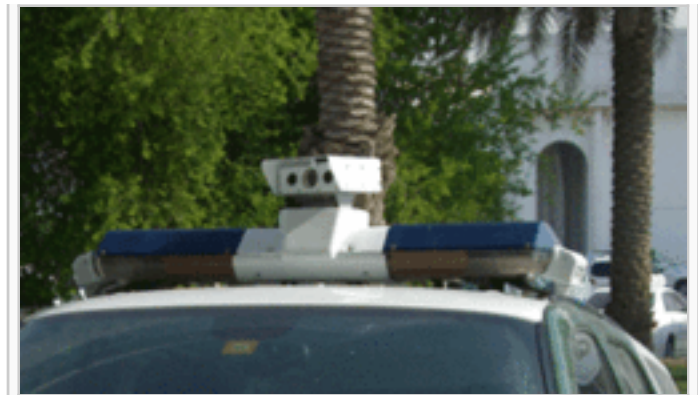
The Dubai police use three Petards ANPR cameras to monitor vehicles in front and either side of the patrol car
