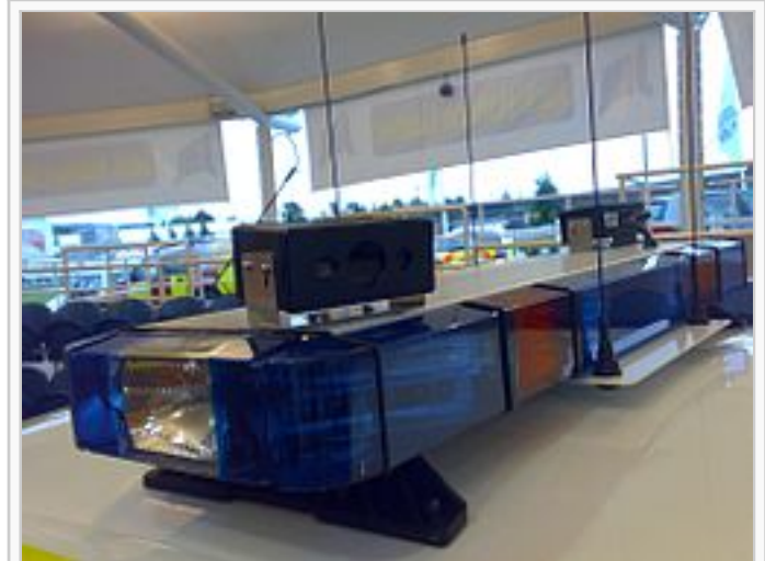
The MiniHawk 2i – one of the most used mobile ANPR cameras in the UK
