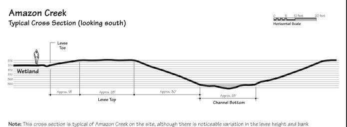
**Note:** This cross section is typical of Amazon Creek on the site, although there is noticeable variation in the levee height and bank slope along its length. The levee has also been breached in several locations. The cross section is based on existing two-foot contour information and measurements taken at a single point along the channel. The cross section will be refined prior to any proposed modifications.
