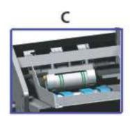
Indexing feed drum quickly rotates without the use of tools or technical adjustment
