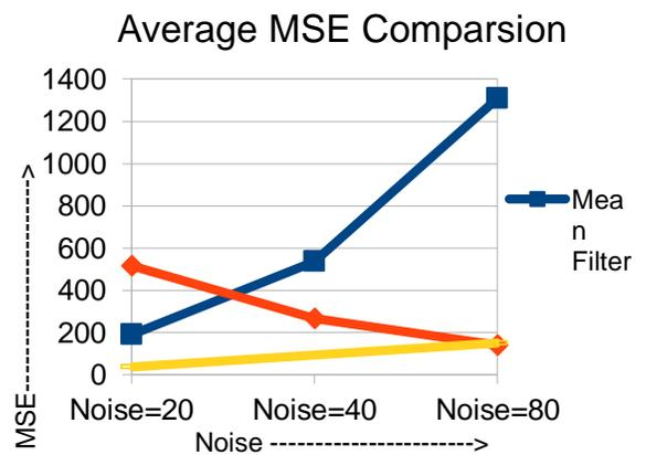
Graph.1.2: Comparison between Mean, Median and adaptive filter MSE
