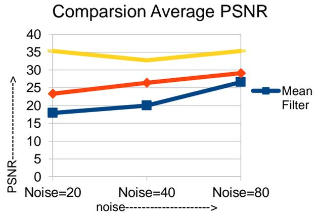
Graph 1.1: Comparison between Mean, Median and adaptive filter PSNR
