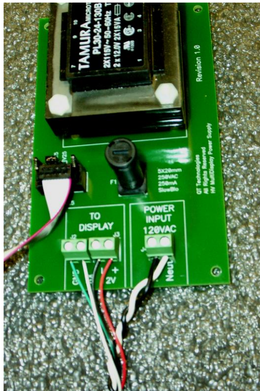
Power Supply Connections
