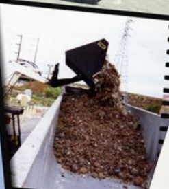
Standard Bucket Dump Height 7'6"
