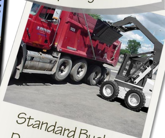
Roll-Out Bucket Dump Height 11'6"
