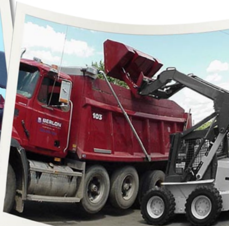
Roll-Out Bucket Dump Height 11'6"
