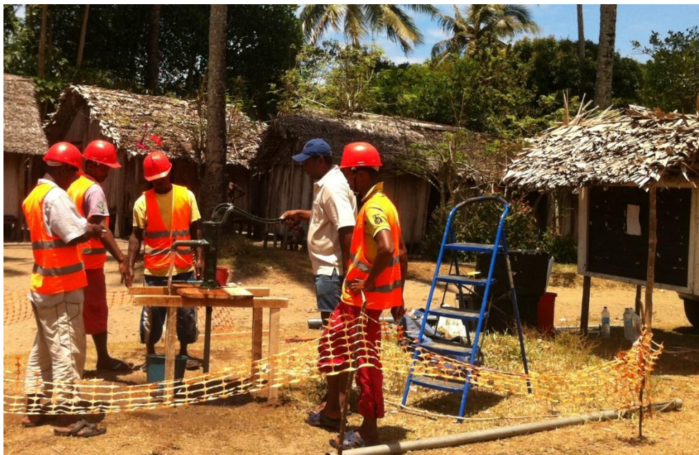
Preliminary well testing of the Andavakimena well
