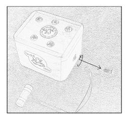
1: Unscrew the bolt at the end of box and detach the mallet.
