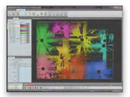
Use up to 128 layers; lock, rename, save, and delete layers easily. Utilize LAS classifications and create layers from clouds.
