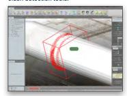
New clash detection tools allow the user to identify clashes between point clouds and point clouds, or point clouds and 3D models.
