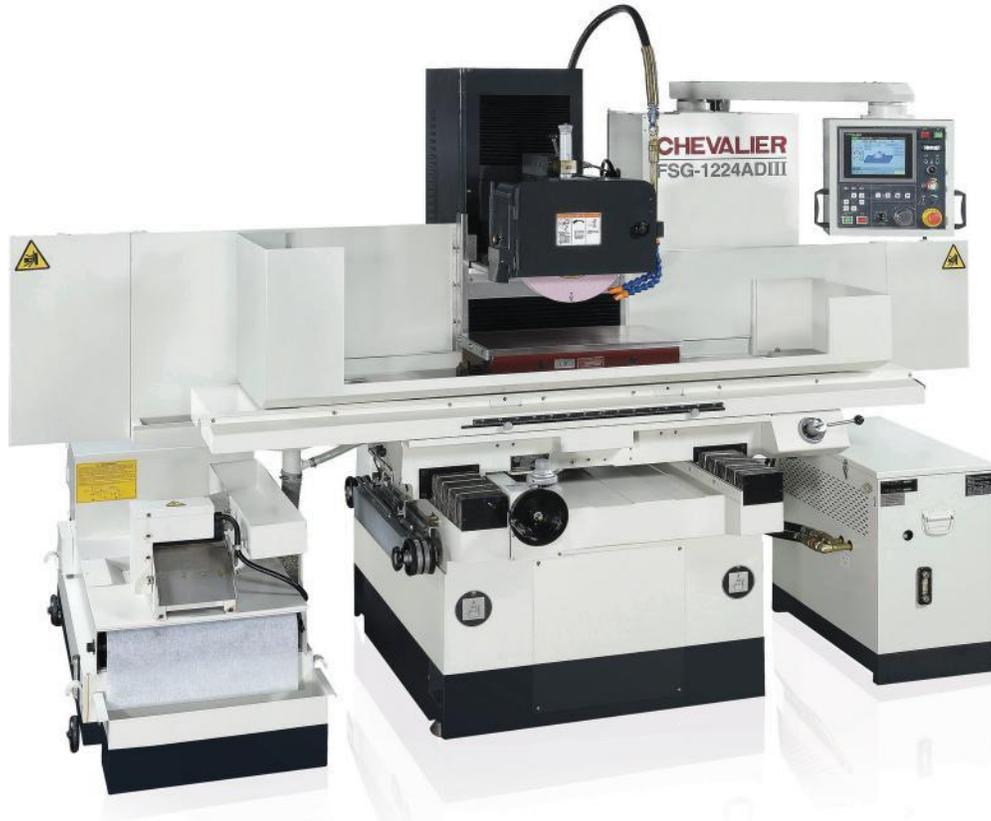
A new feature of the highly rigid construction and stability of the FSG-1224ADIII increases cutting capability. The series features a new PLC controller that includes a grind cycle with rough and fine grinding, spark-out passes and an automatic over-wheel dresser with compensation that can be added to a fully automatic grinding process. After the cycle is finished, the table will "park" either left or right of the saddle and at the front to facilitate unloading and loading.
