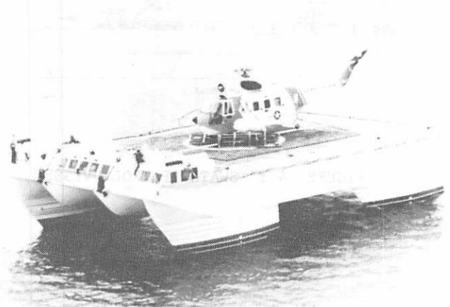
FIGURE 1 : 225 TONNE "KAIMALINO" (U.S. Navy Photograph)
