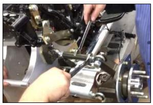
Step 48 Install one Bottom Shock Mount (part #1328), using two 3/8"-16 x 1" Bolts (part #1252) and two 3/8" Lock Washers (part #1254)
