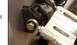
Step 38 Insert one Outer Drive Shaft Assembly (part #1312) onto the bottom on the Control Arm (part #1296)
