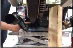
Step 21 Install the Top Mount Assembly, using two 3/8"-16 x 1" Bolts (part #1252), two 3/8" Flat Washers (part #1256), two ½"-13 x 2 ½" Bolts (part #1266), two ½" Lock Washers (part #1262), two Top Mount Plates (part #1268), two 7/8" Top Mount Spacers (part #1270) and one Top Mount Cross Shaft (part #1272)
