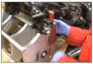
Step 22 Install two 7/16"-14 x 1 ¼" Swing Arm/Main Bolts (part #1274), two 7/16" Lock Washers (part #1276) and two 7/16" Flat Washers (part #1278) to lock Swing Arm and Main Assembly in place
