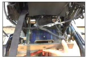
Step 9 Install 1" Spacer (part #1246) onto Swing Arm using a 1/4-20 x 2" Bolt (part #1248) to stabilize brake lines
