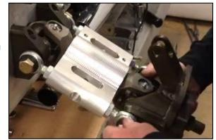
Step 40 Install the bottom Spherical Bearing of the Top Support/Adjusting Tube into the slot on the top of the Outside Carrier (part #1314), using a 5/8"-18 x 2 1/4" Bolt (part #1316), two Spherical Bearing Seals (part #1298) one on either side of the Spherical Bearing and one 5/8" Nylock Nut (part #1318)
