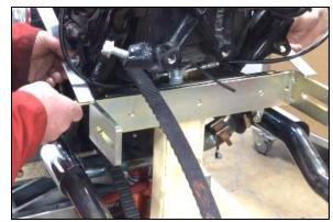
Step 12 Tighten the Adjustable Swing Arm Bolts (part #1252)
