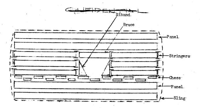
Bridge parts that are contained in this stack are as follows:
