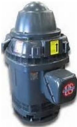
Vertical motors are very unique, they need specific yearly attention. A visual check will not determine bearings, packing or proper alignment of the motor.
