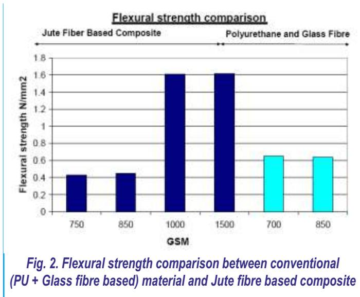
**Fig. 2. Flexural strength comparison between conventional (PU + Glass fibre based) material and Jute fibre based composite**
