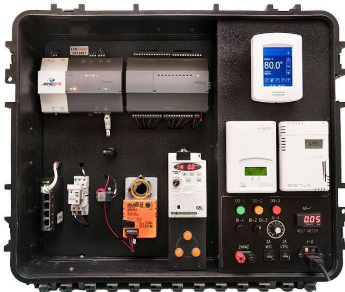
environment. Onboard temperature, CO<sub>2</sub>, humidity, and motion sensors are included. Graphical object oriented programming is presented using the Niagara N4 Framework®. The rugged, weatherproof case has built-in rollers and a retractable handle. The case can be permanently mounted to a tabletop using the integral mounting slots.
