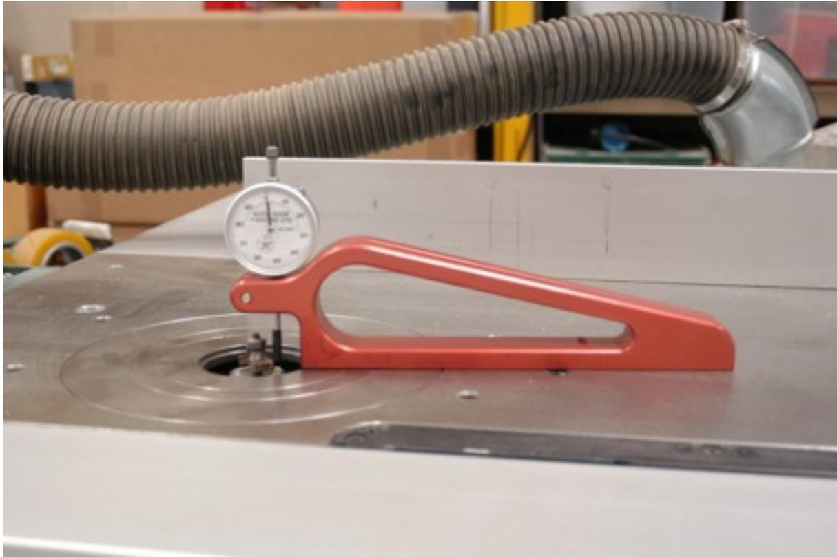
Or without the rings, the base is long enough to not tip into the opening, again, height is limited unless you want to use 1-2-3 blocks to raise it up.
