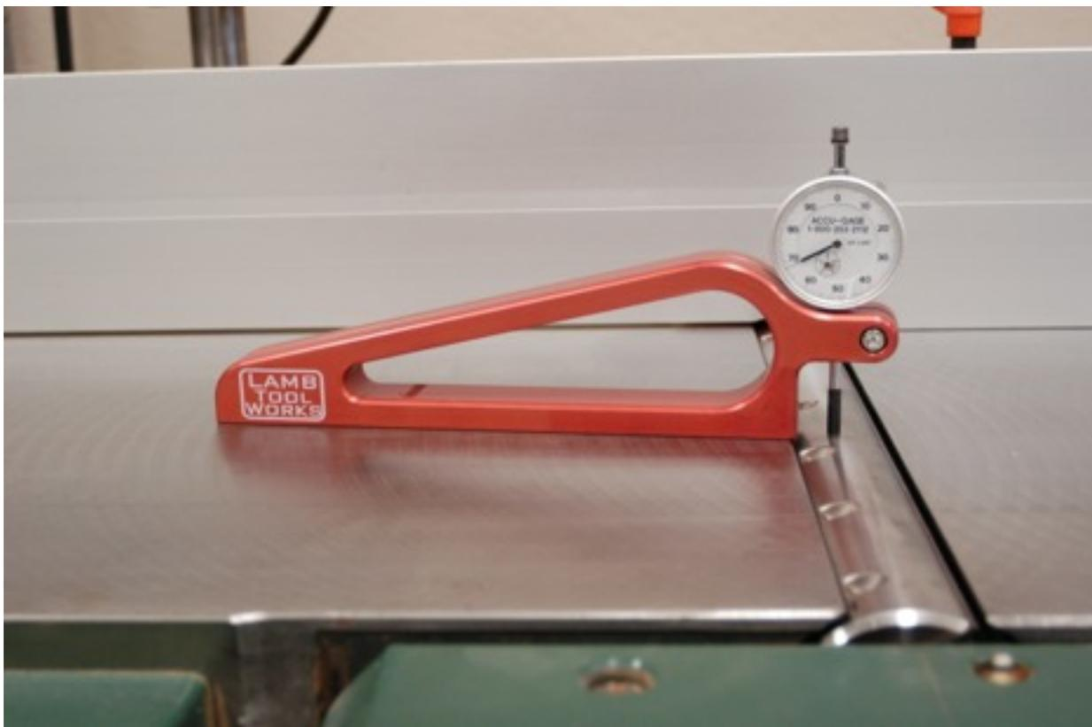
Check the in feed table coplanar to the out feed, far side....
