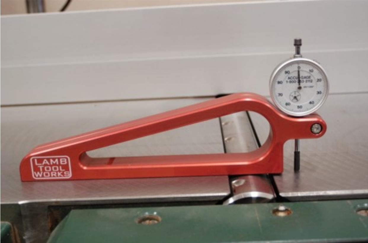
On planers you can check bed rollers, and parallelism of the cutting head to the bed by turning the indicator over and raising the Indicator Holder using 1-2-3 blocks, or even a piece of planed wood, anything parallel and of appropriate height.
