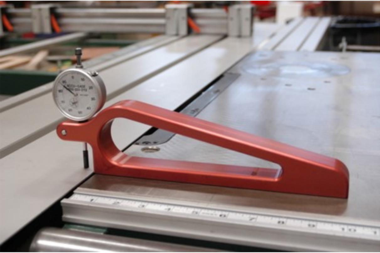
Set router bits or shaper cutter, with the rings...
