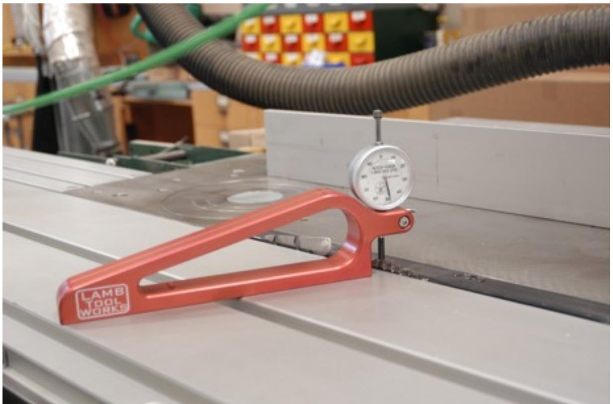
On a sliding table saw you can check height of the slider in relation to the saw table
