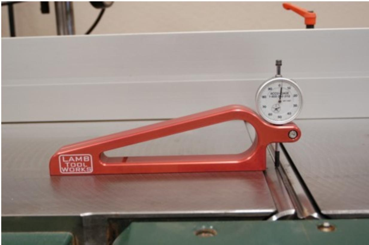
Check the height of the table to the actual cutter head (protrusion of the knives)
