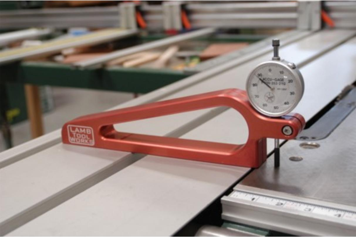
Or check runout of the slider in relation to the saw table
