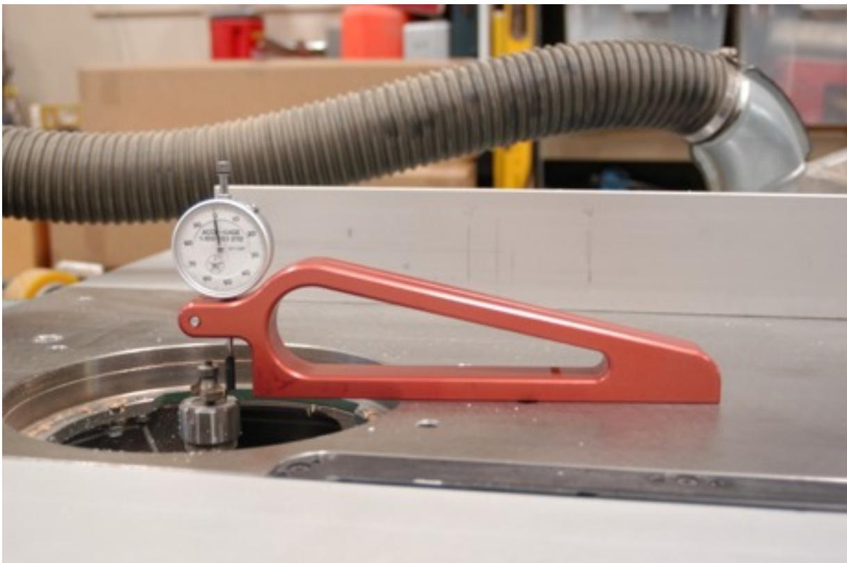
You can do incremental movements of the rip fence. Say you cut something to match another existing part and you find it to be .038" too wide, you can lay the Indicator Holder on it's side and gently slide it to the fence until you get a zero reading. Unlock the fence and use your micro adjust to creep the fence exactly .038" on the dial.
