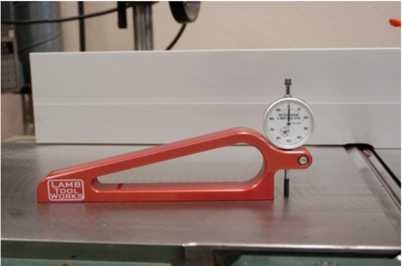
Then you can check blade height side to side in relation to the out feed table
