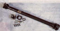
Sturdy Fix: Custom-built double-cardan driveshafts are available from Great Basin Rovers. These solve the vibration problems in the Discovery and are completely serviceable for the DII. Great Basin Rovers also sells a driveshaft service kit to upgrade the D II front driveshaft to fully serviceable if you want to save money and install the parts yourself. Contact: Great Basin Rovers
