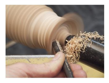
I will return to the inside and continue to shape the interior as much as possible with the tailstock in place. Keeping the tailstock in place reduces the vibration which helps give a better cut especially on longer goblets. For this I will use a 3/8" fingernail grind bowl gouge ground at about 40 degrees, this gives me a bit more clearance working arround the livecenter.
