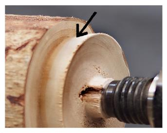
When making a tennon it is critical that the tennon is precisely square for straight jaw chucks or with the correct taper for Dovetail jaw chucks and that the corner is very clean and not rounded (arrow above). The length of the tennon must not be so long as to contact the bottom of the chuck jaws but should allow the face of the jaws to contact the bottom face of the limb. This is critical for the strongest hold and to help eliminate as much vibration as possible. Sharpen your gouge.
