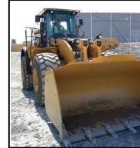
Look for wear on buckets and teeth. Reversible cutting edges are a plus.
