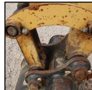
Bearings and bushings should have grease on them. While operating, look for any signs of flex or play.
