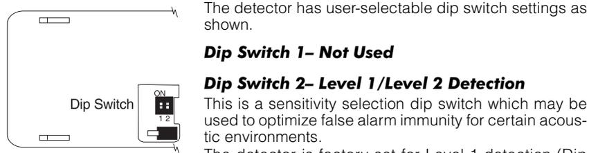
The detector has user-selectable dip switch settings as shown.
