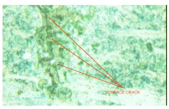
PHOTO No. 17 RUPTURED RISER TUBE "F" MICRO-STRUCTURE
