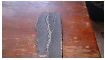
PHOTO No. 30 TENSILE TEST SPECIMEN FAILED DURING MACHINING
