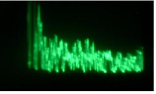
PHOTO No.28 TUBE"E" ECHOES SHOWED LARGE FAILURE
