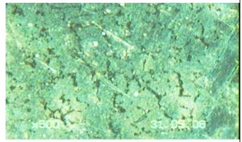
PHOTO No. 14 RUPTURED RISER TUBE "E" MICRO-STRUCTURE
