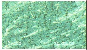
PHOTO No. 12 RUPTURED RISER TUBE "D" MICRO-STRUCTURE
