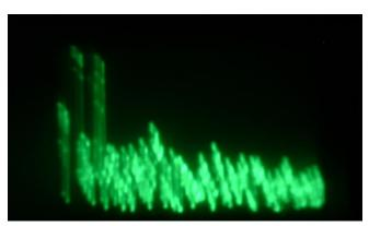
PHOTO No.29TUBE "F" ECHOES SHOWED LARGE FAILURE
