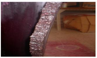
PHOTO No. 3 RUPTURED TUBE "A" SECTION
