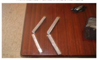
BEND TEST SPECIMENS FAILED SHOWING BRITTLE NATURE FRACTURE
