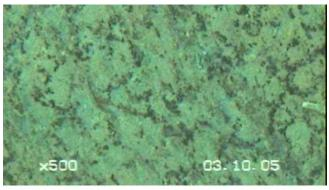
PHOTO No. 7 RUPTURED RISER TUBE "A" MICRO-STRUCTURE
