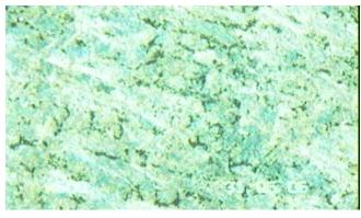
PHOTO No. 11 RUPTURED RISER TUBE "C" MICRO-STRUCTURE
