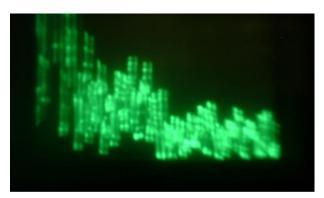
PHOTO No.26TUBE "C" ECHOES SHOWED MODERATE FAILURE
