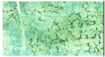
PHOTO No. 16 RUPTURED RISER TUBE "F" MICRO-STRUCTURE
