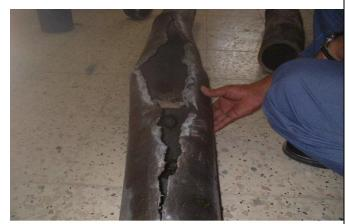
PHOTO No. 2 RUPTURED TUBE "A"
