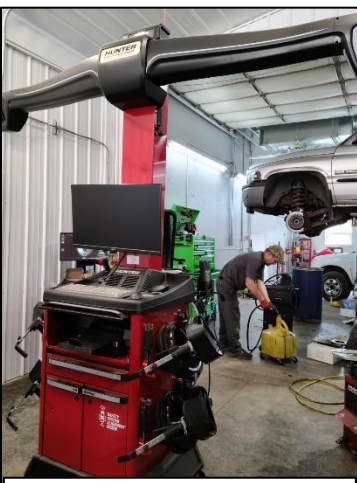
Alignment system in the new service bay
