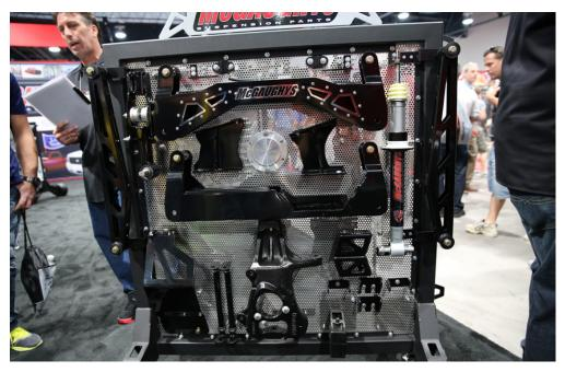
On the lighter side of things, they were showing off their 2014 1500 Chevy and GMC 7- to 9-inch lift kit. These kits actually fully drop the differential seven inches to maintain factory geometry while supplying all of the parts necessary to install the kit.
