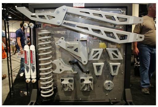
For the 2011-2013 Ford Super Duty with four-wheel drive, McGaughys Suspension has just recently introduced their new phase 3-lift kit. The phase three lift kit is a true 8-inch lift. All of the components are fully boxed with interlocking pieces to ensure proper fitment.
