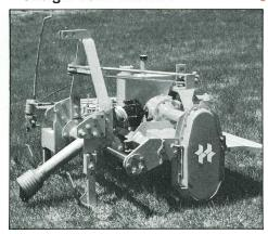
The key is hydraulics and an adjustable "feeler arm" which gently touches a plant or obstacle in a row, retracts the ROTAVATOR toward the tractor, then lets it offset again when the obstacle is past. Interplant tillage was never easier, never faster or more complete.
