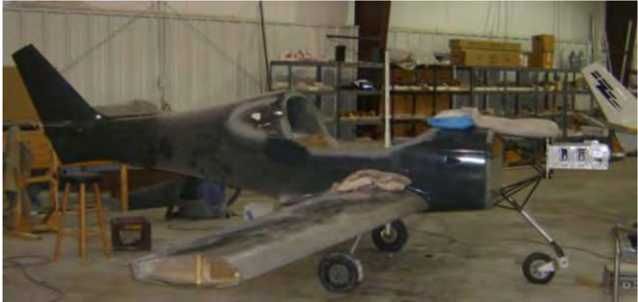
Lightning Sport “drop test” rig with deflection rod in place.
