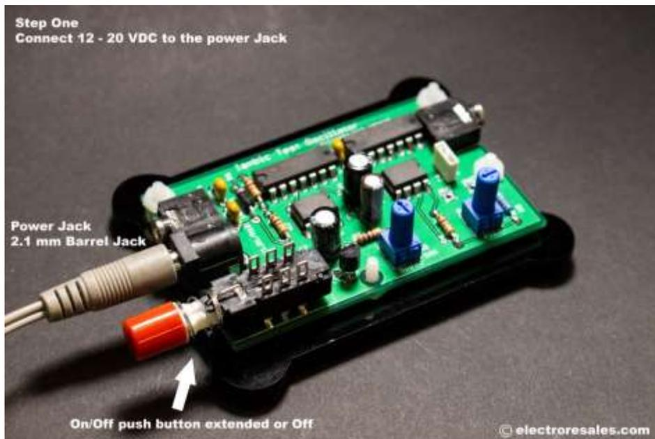
Next attach the Iambic paddle, if your paddle connects using a jack plug using a standard stereo 3.5mm to 3.5mm jack cable the paddle will be operating in what is referred to as Normal Iambic, where the dot is generated by the left hand paddle. If your paddle has screw terminals then a cable may need to be constructed, see the appendix for help on this.
